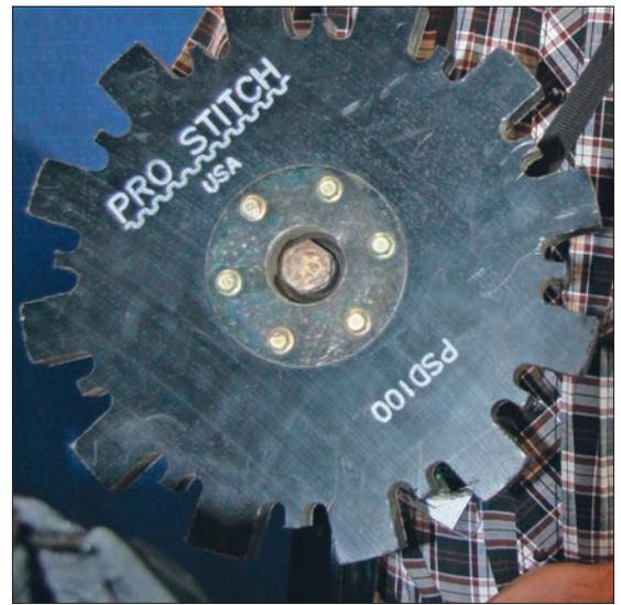
The unique, toothed circumference on the Pro-Stitch closing wheel is able to seal up the seed trough in muddy conditions without compacting the soil.
