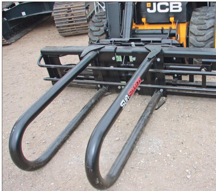
The Sure-Squeeze from MDS in South Dakota can lift up to 4,400 pounds, depending on tractor capacity. It's designed to handle big tires as well as bales. It lists for US\$4,850 without a mounting kit. There are mounting kits for more than 90 different tractors and loaders, all in the \$1,000 price range. | RON LYSENG PHOTOS
