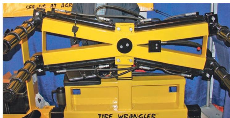
The Tire Wrangler uses two arms on each side to stabilize large diameter tires and prevent them from slipping out.
